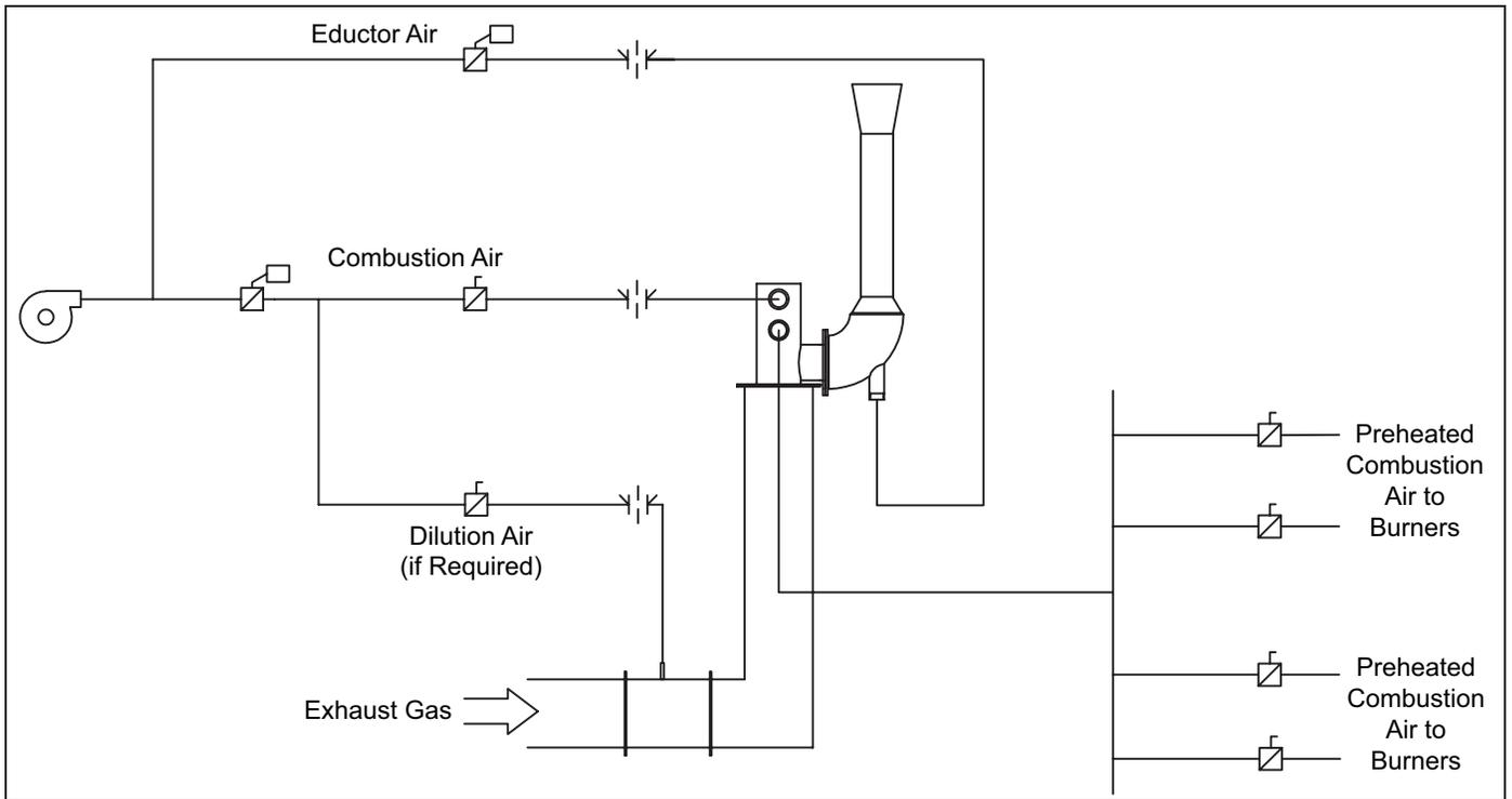
Figure 3.5. P & ID of Typical Piping for Greater Furnace Pressure Control
